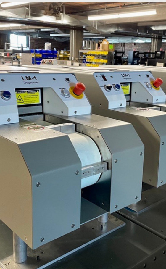
Degausser machines at Data Security Inc.® Degaussers magnetically randomize the 0's and 1's so that data cannot be put back together and deciphered.
